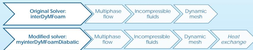
An existing solver, *interDyMfoam*, has been used as a basis for this project. The figure shows physical phenomena that are taken into account for the original solver and modified one. Heat exchange has been introduced adding two main features: computation of temperature field and temperature dependent fluid properties such as viscosity and density.
