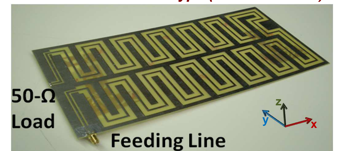
Snake Antenna Prototype ( 275 \times 135 mm 2 )
